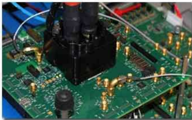
Figure 1: Active thermal management system
