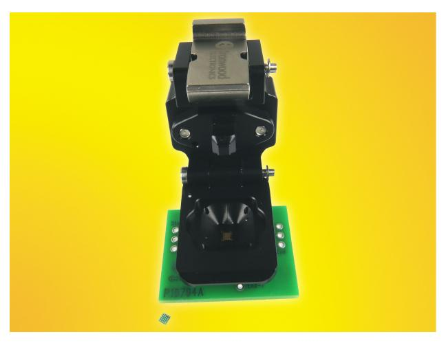
The CG-BGA-5030 socket is constructed with high performance and low inductance elastomer contactor. The temperature range is -35 °C to +125 °C. The pin self inductance is 0.11 nH and mutual inductance of 0.028 nH. Capacitance to ground is 0.028 pF. Current capacity is 2 amps per pin.
