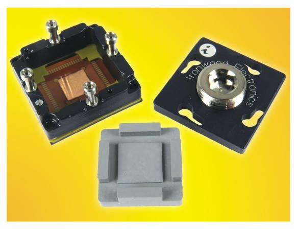
The SG-QFE-7011 sockets are constructed with high performance and low inductance gold plated <a href="embedded wire">embedded wire</a> on elastomer as interconnect material between device and PCB. It also has a square copper foil in the middle to connect the ePad which is at different plane than the peripheral leads. The temperature range is -35C to +125 C. The pin self inductance is 0.15 nH and mutual inductance of 0.025 nH. Capacitance to ground is 0.01 pF. Current capacity is 2 amps per pin.
